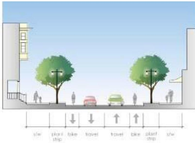
Figure 4.8—Collector Street Section without Parking
